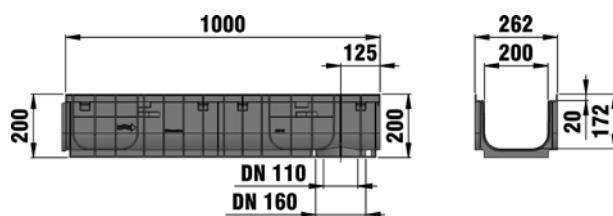
Type 115 with FIBRETEC design slotted grating, SW 9 mm, black, locked
