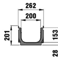
Type 115 with longitudinal ductile iron grating SW 9 mm, KTL-coated, locked
