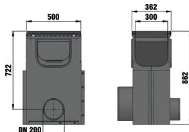
Trash box with galvanised mud bucket and G-TEC Ductile iron grating, SW 2 x 141 x 9 mm, KTL-coated, class C 250, locked, with PVC-U pipe outlet DN/OD 200
