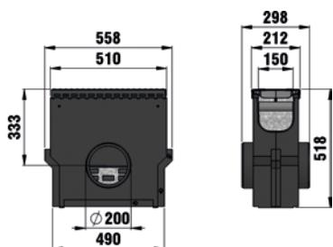
Trash box with galvanised mud bucket and FIBRETEC design slotted grating, black, SW 9 mm, class B 125, locked
