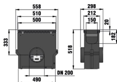
Trash box with galvanised mud bucket and longitudinal ductile iron grating SW 9 mm, KTL, class C 250, locked
