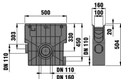
Trash box with PE mud bucket and slotted grating SW 80/10 mm, class A 15, locked
