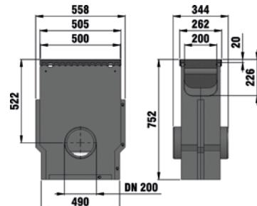
Trash box with galvanised mud bucket and FIBRETEC design slotted grating, SW 9 mm, black, class B 125, locked
